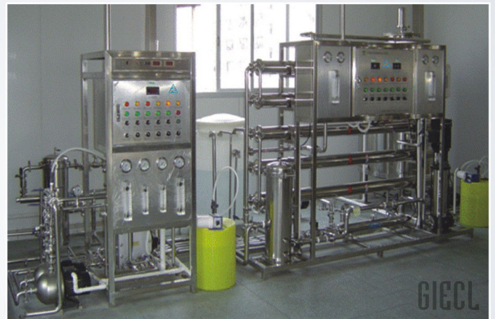
2.0 M3/Hr HSRO System with EDI system for Ultra High Purity Water for Pharmaceutical industries for USP, EP, WFI standard
