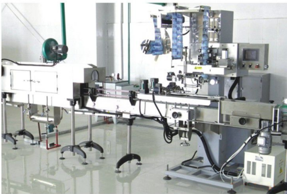
6000 BPH Automatic PVC Shrink Sleeve Applicator with Steam Tunnel for PET / Glass Bottles for Labeling
