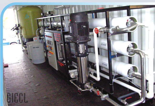
15.0 M3 / Hr. Brackish Water containerize R.O. system for Mobile transportation and use at Island for city council supplies
