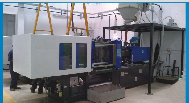
Injection Molding machine for PET preform and Cap Closure manufacturing for Soft-drink, Juice and PET water Bottle production
