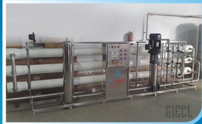
15.0 M3 / Hr. R.O. System for Industrial use for Utility requirement such as Boiler, Cooling Tower, Laundry ect..
