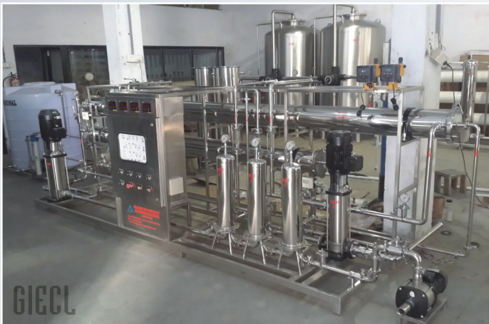
3.0 M3/Hr Two Pass R.O. System with Ultra Pure water production for Pharmaceutical factory
