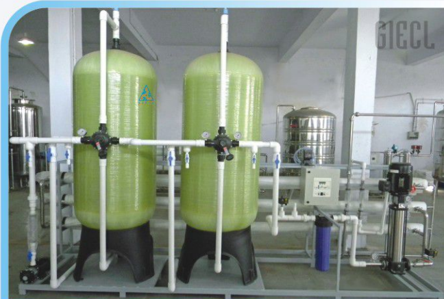
3.0 M3/Hr. R.O. System with Filtration, U.V. System for Drinking water in Institution, Hospital, Soft Drink, Juice, Bakery application
