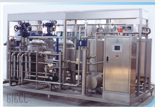
Pasteurization system for Hot-fill Juice Processing with Pulp, Fibers, enzymes for Orange, Mango, Apple, Mix fruit
