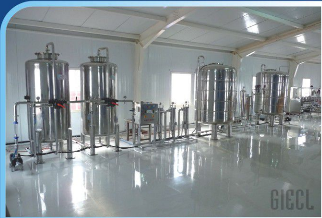
12.0 M3/Hr Spring Water Filtration System complete in Sanitary type S.S. 316L material for High Grade Bottled water
