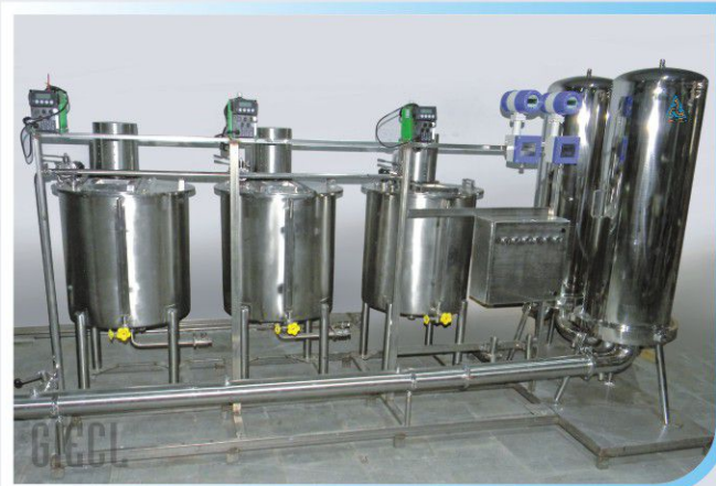
Fully Automatic Sanitary type Online Mineral Adding system for High Purity Bottled Drinking water using online taste controller and operation with pH and TDS meter with 1 micron and 0.2 Micron Fine Filtration followed by UV system complete in SS 316
