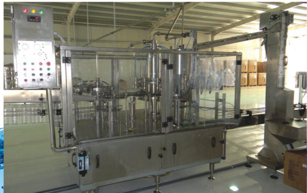
4,800 BPH - 24,000 BPH High Speed Fully Automatic Rotary 3 in 1 Rinsing Filling/Capping machine with Cap Hopper and Loader with Online Cap Washing Air Exhaust Filling system with No Bottle Rinse - Fill System
