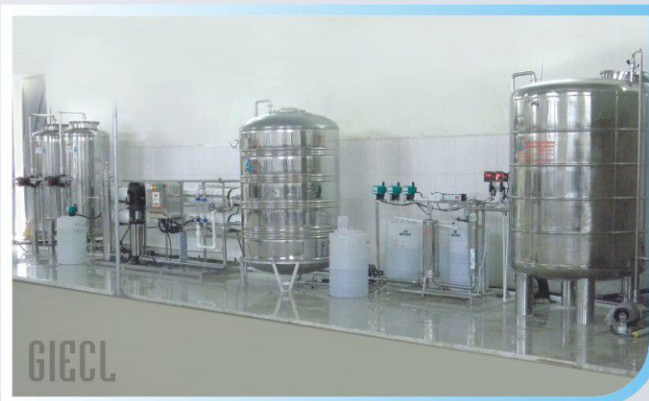
6000 LPH R.O. System for Mineral Water Industries complete in S.S. 316 with Online Mineral Adding System for different taste of Bottled water
