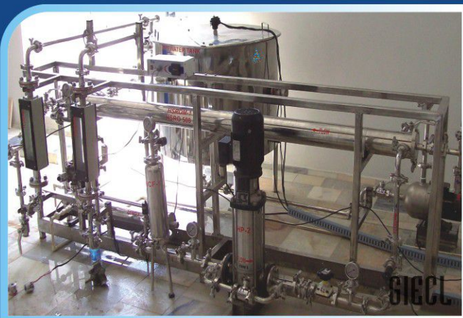
1.5 m3/ hr. HSRO ( Hot Water Sanitisable) system for Pharmaceutical Industries
