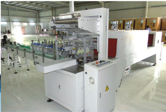
Fully automatic 10 - 30 packs per Minute Automatic Shrink Group packing machine with or without tray, hard Board
